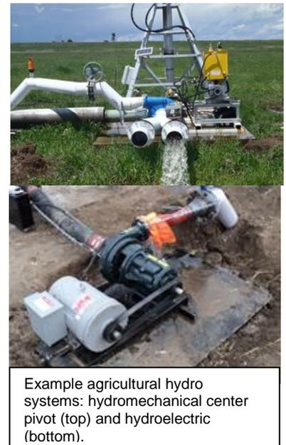
Example agricultural hydro systems: hydromechanical center pivot (top) and hydroelectric (bottom).
